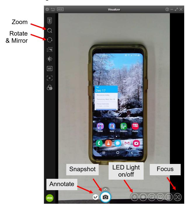
**Snapshot** – Take a picture of what the camera is displaying **Annotate** – Draw pictures on the computer screen using your mouse.
