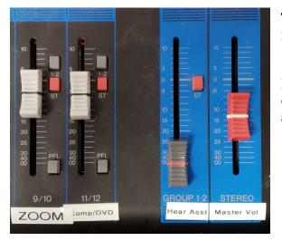
To control the volume for the entire sound system, use the red Master Vol slider on the AV system.
